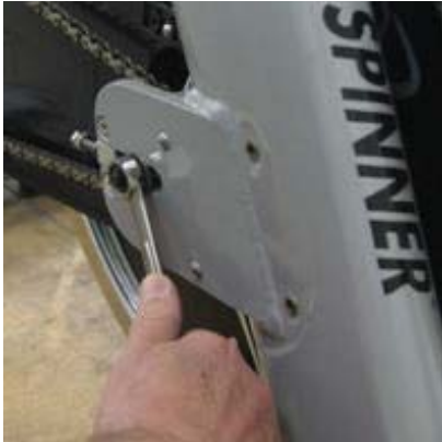
Tighten the nut to 30 lbs-ft
