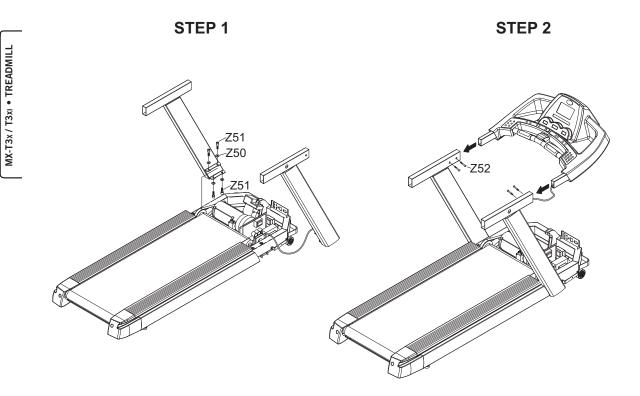
Remove the motor cover. Pull out the console cable and route it through the Right console mast. Place the right console mast and then the left console mast in the console post support brackets. Secure the Right and Left mast with the 4 bolts provided (Z50, Z51). Make sure these bolts are tight.
