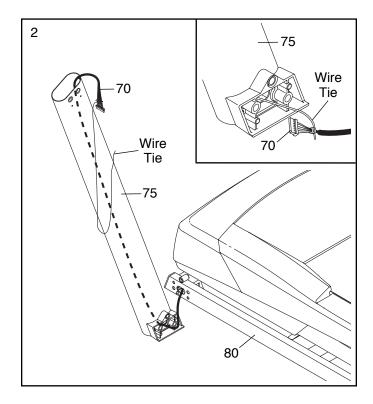
Hold the Left Upright (75) against the Base (80). Be careful not to pinch the wires.
