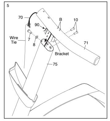
6. Remove the tie from the 5/16" Cage Nut (90). If necessary, press the Cage Nut back into place.
