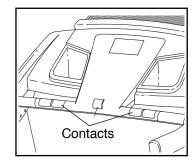
To measure your heart rate, stand on the foot rails and hold the metal contacts on the handrails for approximately ten seconds—avoid moving your hands. When your pulse is detected, a heart symbol in the calorie display will flash each time your heart beats, one or two dashes will appear, and then your heart rate will be shown. For the most accurate heart rate reading, continue to hold the contacts for about 15 seconds.
