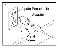
The lug or wire extending from the adapter must be connected with a metal screw to a permanent ground such as a properly grounded outlet box cover. Some 2-pole receptacle outlet box covers are not grounded. Before using an adapter, contact a qualified electrician to determine whether the outlet box cover is grounded. The temporary adapter should be used only until a properly grounded outlet can be installed by a qualified electrician.
