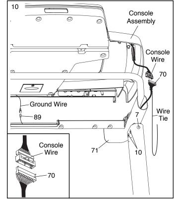
11. Set the console assembly on the Left and Right Handrails (71, 72). Make sure that no wires are pinched. Insert the excess Upright Wire (not shown) into the Left Handrail and the ground wires (not shown) into the console assembly.
