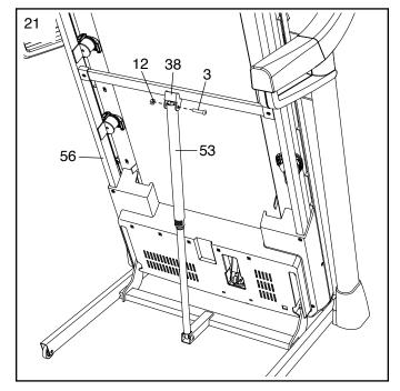
22. Make sure that all parts are properly tightened before you use the treadmill. If there are sheets of plastic on the treadmill decals, remove the plastic. To protect the floor or carpet, place a mat under the treadmill. Note: Extra parts may be included. Keep the included hex keys in a secure place; one of the hex keys is used to adjust the walking belt (see pages 31 and 32).
