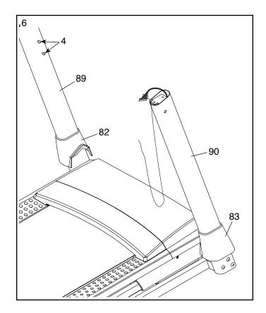
7. Identify the right handrail assembly (B).
