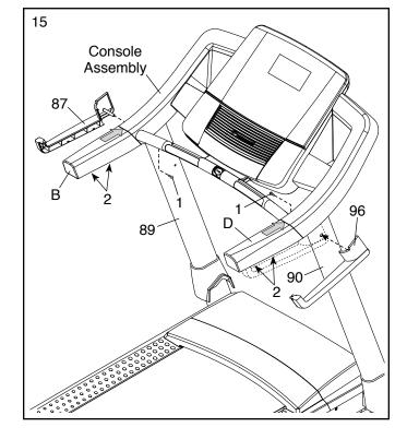
16. Tighten a #8 x 3/4" Screw (2) into the Left Outside Upright Cover (87) and into the bottom of the left handrail assembly (D). Make sure not to overtighten the Screw.
