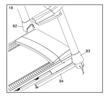
19. Note: If assembled on a smooth surface, the treadmill may roll forward during this step.
