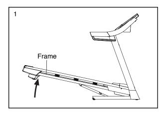
Raise the frame until the storage latch locks in the storage position. CAUTION: Make sure that the storage latch locks.
