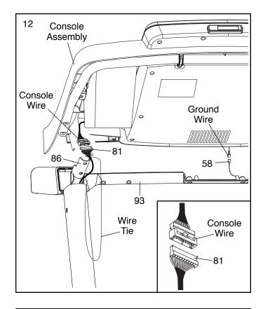
13. Set the console assembly on the brackets on the Handrails (86). Make sure not to pinch any wires. Insert the excess Upright Wire (81) into the Right Upright (90).
