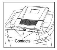
To measure your heart rate, stand on the foot rails and hold the pulse bar with your palms on the metal contacts; avoid moving your hands. When your pulse is detected, a heart symbol in the calorie display will flash each time your heart beats, one or two dashes will appear, and then your heart rate will be shown. For the most accurate heart rate reading, continue to hold the contacts for about 15 seconds.
