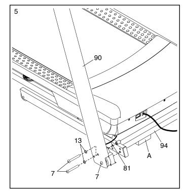
Remove the four indicated 5/16" x 3/4" Screws
