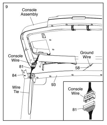
10. Set the console assembly on the Right and Left Handrails (84, 85). **Make sure that no wires are pinched.** Insert the excess Upright Wire (81) into the Right Upright (90).
