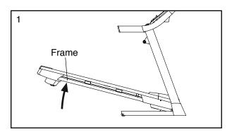
2. Hold the frame firmly with your right hand. Pull the latch knob to the left and hold it. Raise the frame until the latch plate is aligned with the latch pin. Then, slowly release the latch knob; **make sure that the latch pin is resting on the latch plate.**
