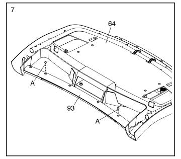
IMPORTANT: To avoid damaging the Pulse Crossbar (93), do not use power tools and do not overtighten the #10 x 1 1/2" Screws (9).
