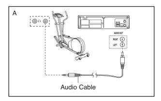
B. Plug one end of a long 1/8" to RCA stereo audio cable (available at electronics stores) into either jack on the console. Plug the other end of the cable into an RCA Y-adapter (available at electronics stores). Next, remove the wire that is currently plugged into the AUDIO OUT jack on your VCR and plug the wire into the unused side of the Y-adapter. Plug the Y-adapter into the AUDIO OUT jack on your VCR.
