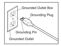
current to reduce the risk of electric shock. This product is equipped with a cord having an equipment-grounding conductor and a grounding plug. Plug the power cord into an appropriate outlet that is properly installed and grounded in accordance with all local codes and ordinances. This product is for use on a nominal 120-volt circuit. Important: The elliptical exerciser is not compatible with GFCI-equipped outlets.
