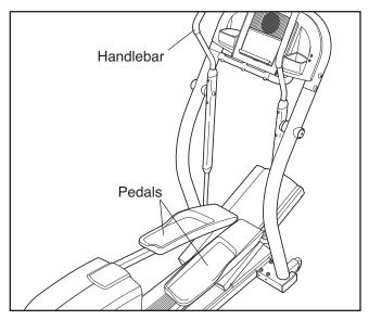
To dismount the elliptical exerciser, wait until the pedals come to a complete stop. The elliptical exerciser does not have a free wheel; the pedals will continue to move until the flywheel stops. When the pedals are stationary, step off the highest pedal first. Then, step off the lowest pedal.
