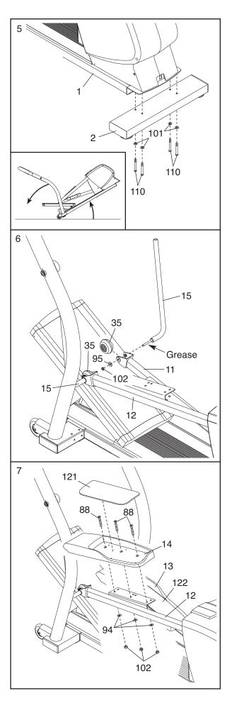
8. Apply a thin film of the included Teflon® lubricant to both Pivot Shafts (15).
