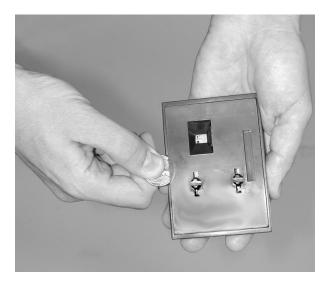
Next, turn the 1154 watch batteries so the positive (+) sides are facing up and insert them into the battery clips. Snap the monitor back together.
