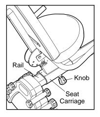
to loosen it (if the knob is not loosened enough, it may scratch the rail). Next, pull the knob, slide the seat carriage to the desired position, and then release the knob. Move the seat carriage back and forth slightly until it locks into position. Then, turn the knob clockwise until it is tight.
