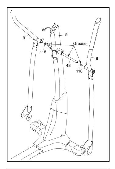
8. At the same time, tighten an M8 x 16mm Screw (102) and an M8 x 23mm x 1.5mm Washer (126) into each end of the Upright Axle (48). Firmly tighten the Screws.
