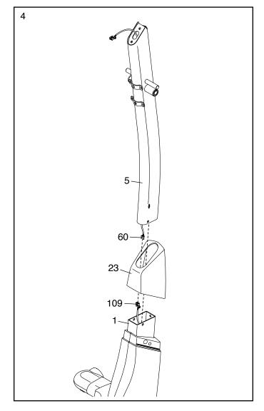
5. **Tip: Avoid pinching the wires.** Insert the Upright (5) into the Frame (1).
