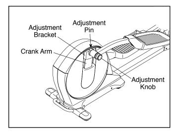
Slide the adjustment bracket upward or downward until the adjustment knob is aligned with one of the holes in the crank arm, and gently release the knob to engage the adjustment pin in the hole.
