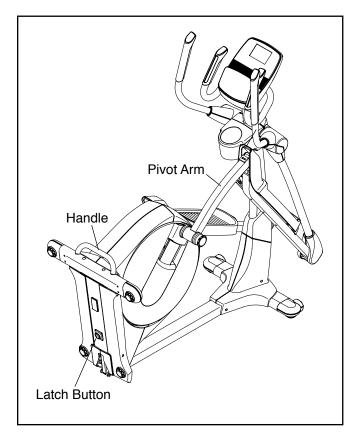
To use the elliptical, first hold the handle, pull back on the frame, press the latch button, and lower the frame.
