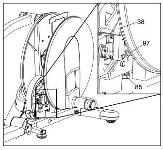
When the Drive Belt (38) is tight, tighten the Pivot Screw (97).
