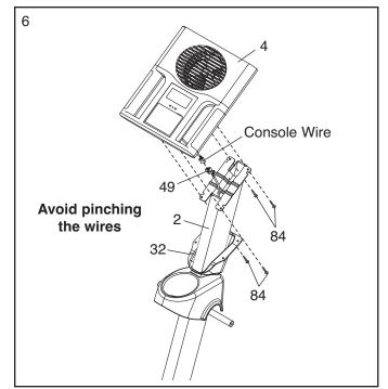
7. Slide the Console Cover (32) (see the drawing in step 6) upward to the Console (4). Attach the Console Cover with four M4 x 16mm Round Head Screws (94).
