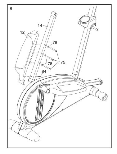
Identify the Left Upper Body Arm (8), which is marked with a "Left" sticker. Orient the Left Upper Body Arm and the left Upper Body Leg (6) as shown; make sure that the hexagonal holes are in the indicated location.
