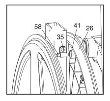
slightly closer to or away from the Magnet, and then retighten the Screw. Rock the Left Pedal Disc forward and backward just enough that the Magnet passes the Reed Switch repeatedly. Repeat until the console displays correct feedback. When the Reed Switch is correctly adjusted, reattach the side shields. Note: If you have questions as to which screw should be in which hole, see EXPLODED DRAWING B on page 23 and the PART LIST on page 21.
