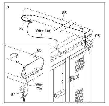
Hold the Right Upright (85) against the Base (95). Be careful not to pinch the Upright Wire (87). Insert two 3/8" x 4" Screws (7) with two 3/8" Star Washers (11) and a 3/8" x 1 1/2" Screw (14) with a 3/8" Star Washer (11) into the Right Upright.
