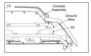
14. Set the console assembly on the Left and Right Handrails (82, 83). **Be careful not to pinch any wires.** Insert the excess Upright Wire (87) into the Right Handrail.
