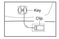
the console. After a moment, the displays will light. IMPORTANT: In an emergency, the key can be pulled from the console, causing the walking belt to slow to a stop. Test the clip by carefully taking a few steps backward; if the key is not pulled from the console, adjust the position of the clip.
