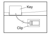
displays will light. IMPORTANT: In an emergency, the key can be pulled from the console, causing the walking belt to slow to a stop. Test the clip by carefully taking a few steps backward; if the key is not pulled from the console, adjust the position of the clip. Note: The first time you insert the key into the console, the incline may automatically rise to the maximum incline level and then return to the minimum incline level.
