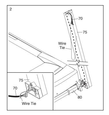
3. Hold the Left Upright (75) against the Base (80). Be careful not to pinch the Upright Wire (70). Partially tighten three 3/8" x 3 1/2" Screws (4) with three 3/8" Star Washers (5) into the Left Upright and the Base; do not fully tighten the Screws yet.
