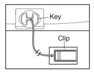
light. IMPORTANT: In an emergency, the key can be pulled from the console, causing the walking belt to slow to a stop. Test the clip by carefully taking a few steps backward; if the key is not pulled from the console, adjust the position of the clip. Note: The first time you insert the key into the console, the incline may automatically rise to the maximum incline level and then return to the minimum incline level.
