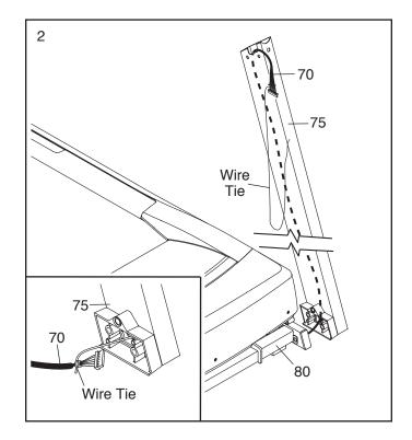
3. Hold the Left Upright (75) against the Base (80). **Be careful not to pinch the wires.** Partially tighten three 3/8" x 3 1/2" Screws (4) with three 3/8" Star Washers (5) into the Left Upright and the Base; **do not fully tighten the Screws yet.**
