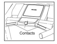
When your pulse is detected, a heart symbol in the calorie display will flash each time your heart beats, one or two dashes will appear, and then your heart rate will be shown. For the most accurate heart rate reading, continue to hold the contacts for about 15 seconds.
