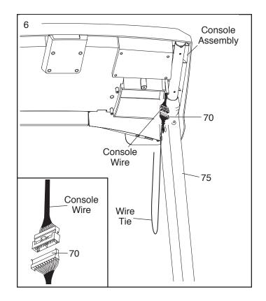
7. Insert the Upright Wire (70) into the Left Upright (75) as you set the console assembly on the Left Handrail (71) and the Right Handrail (72). **Make sure that no wires are pinched.**
