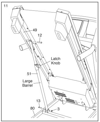
12. Make sure that all parts are properly tightened before you use the treadmill. If there are sheets of plastic on the treadmill decals, remove the plastic. To protect the floor or carpet, place a mat under the treadmill. Note: Extra hardware may be included. Keep the included hex key in a secure place; the hex key is used to adjust the walking belt (see pages 24 and 25).
