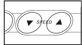
To stop the walking belt, press the STOP button. The TIME display will begin to flash. To restart the walking belt, press the START button or the SPEED  $\Delta$  button.
