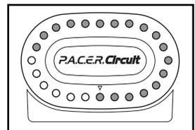
**DISTANCE/INCLINE/LAPS display**—This display shows the distance that you have walked or run, the incline level of the treadmill, and the number of laps you have completed (one lap equals 1/4 mile). The display will change from one number to the next every seven seconds, as shown by the indicators beside the display.
