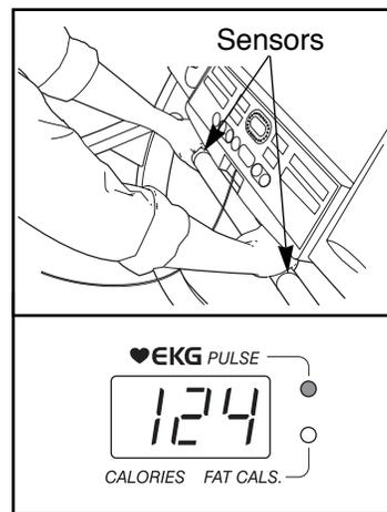
When your pulse is detected, the indicator above the CALS./FAT CALS./PULSE display will light and a series of dashes (— —) will appear. Your heart rate will be shown. **For the most accurate heart rate reading, continue to hold the contacts for about 15 seconds.**
