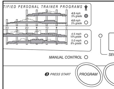
The console features two low intensity programs, two medium intensity programs, and two high intensity programs. The profiles on the console show how the speed and incline of the treadmill will change during the programs. The numbers beside the profiles show the maximum speed and incline settings for the programs. For example, the upper left profile shows that the treadmill will reach a maximum speed of 4.5 mph and a maximum incline of 5% during the first program.
