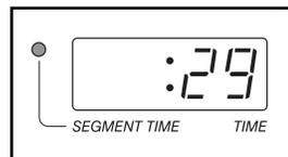
One speed setting and one incline setting are programmed for each segment. When only three seconds remain in the first segment, a series of tones will sound and the treadmill will automatically adjust to the speed and incline settings for the second segment.
