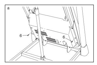
Lower the treadmill. Next, remove the three indicated #8 x 3/4" Screws (6). Carefully slide the Motor Hood (57) off.
