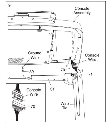
Set the console assembly on the Left and Right Handrails (71, 72). Make sure that no wires are pinched. Insert the excess Upright Wire (70) behind the Console Frame (87).
