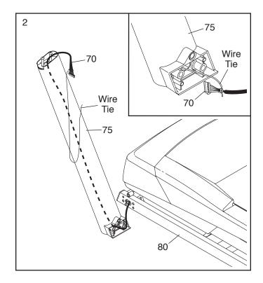
3. Hold the Left Upright (75) against the Base (80). Be careful not to pinch the wires. Partially tighten three 3/8" x 4" Screws (4) with three 3/8" Star Washers (5) into the Left Upright and the Base; do not fully tighten the Screws yet.
