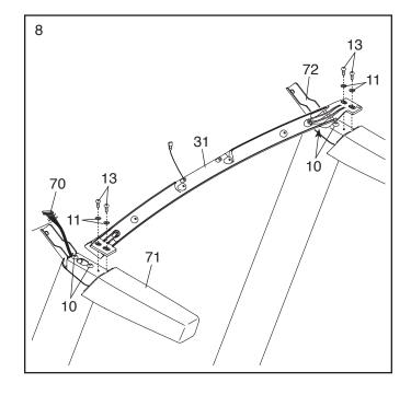
9. With the help of a second person, hold the console assembly near the Left Handrail (71) and the Right Handrail (not shown).
