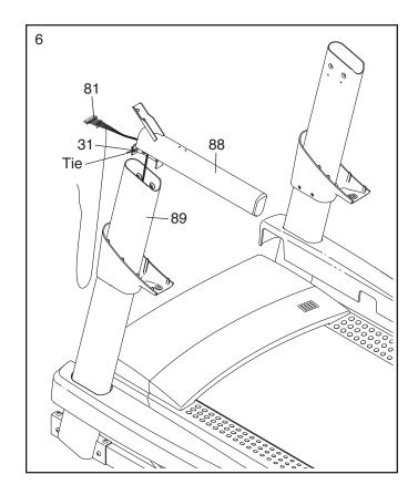
7. Attach the Left Handrail (88) to the Left Upright (89) with two 5/16" x 1" Bolts (5), two 5/16" Star Washers (11), and a 5/16" x 1 1/4" Bolt (4). **Do not fully tighten the Bolts yet.**
