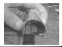
6) Finally loop ribbon cable over and plug into the back of the upper display board.
