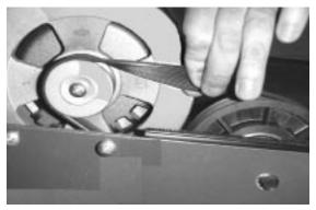
The proper twist is 45°. If the belt needs to be adjusted use a 7/16" socket and turn the bolt underneath the motor pan attached to the hook screw.
