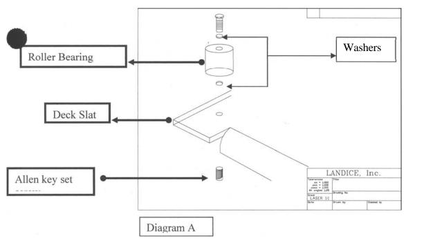
These roller guides are almost silent in forward position, but may be heard in the reverse position. The roller guides should spin freely. Loosen the set screw with a 10/32 allen key until the roller guide to spins freely.
