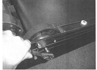
Lift deck out of treadmill frame assembly.
