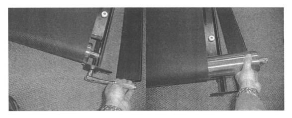
9. Remove front drive-roller; (1/2" hex head bolts on right and left side).
