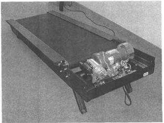
Here is a picture of the treadmill frame with the upright assembly removed.
