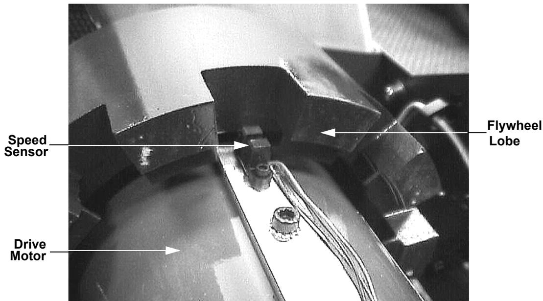
2. If the voltages in step 1 are correct, go to step 5. If the voltage in step 1 is 0 Vdc or significantly low when a flywheel lobe is between the speed sensor "legs", continue with step 3.
