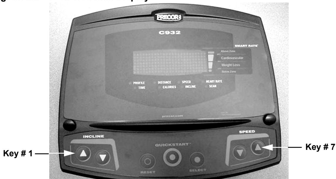
32. The display will scroll **KEYBOARD TEST**. The display will have a representation of every key on the keyboard including the **STOP** key. Press each key on the keyboard to ensure that all keys are functioning normally. Tug on the safety key lanyard, to ensure that the **STOP** key will activate.
