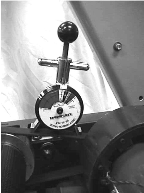
4. The gauge should read approximately 80 inch/pounds. The drive belt tension is acceptable if it is in the range of 70 to 90 inch-pounds.
