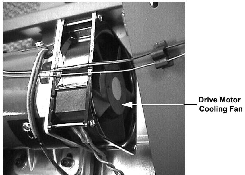
5. Set the replacement drive motor cooling fan at it's mounting position on the drive motor and fasten it with the hardware removed in step 4. Torque the mounting screws to 25 inch pounds.
