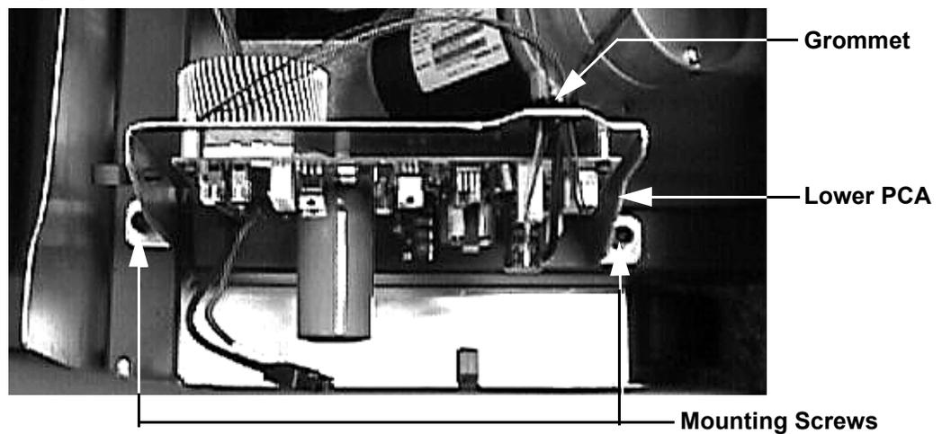
4. Set the replacement lower PCA in its mounting position and fasten it with the screws removed in step 3. Torque the lower PCA mounting screws to 120 inch pounds.
