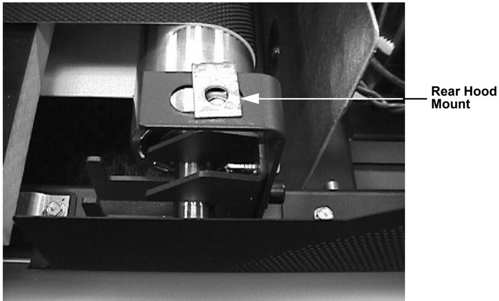
5. Set the replacement hood in its mounting position. Using a thin bladed screwdriver or similar tool into one of the rear hood mounting holes and use the screw driver to align the hood mounting nut with the hole in the hood. Hand start one of the rear hood mounting bolts.
