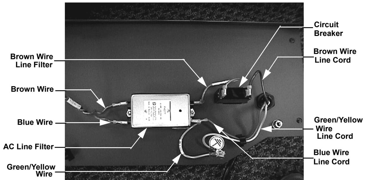
3. Disconnect both brown wires from the circuit breaker.
