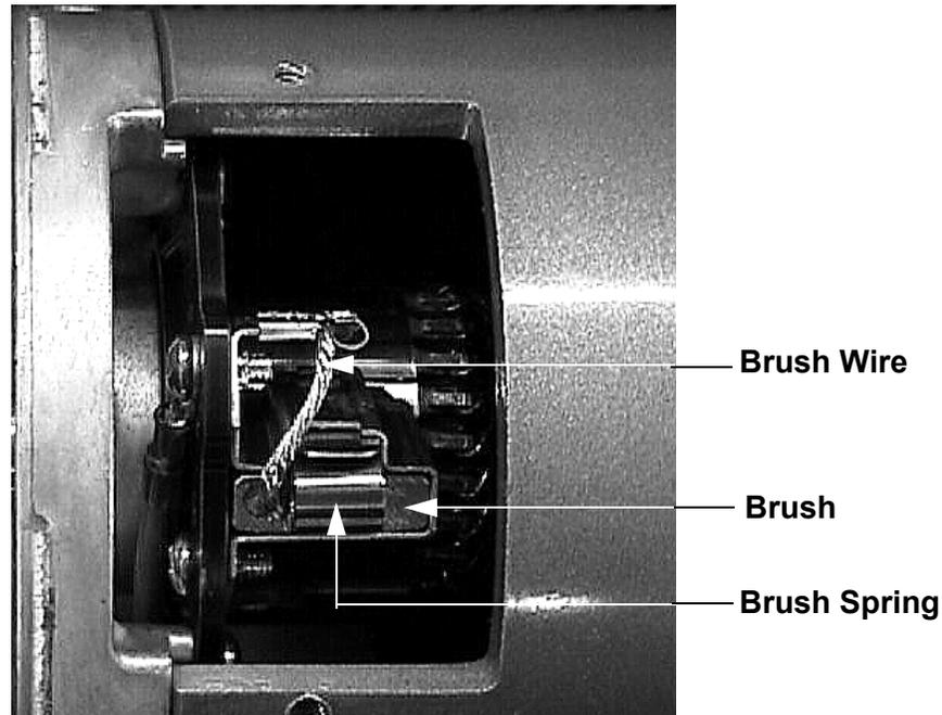
5. Slide the replacement brush into the brush holder. Be sure that the angled edge of the brush is oriented so that the brush face makes full contact with the motor commutator.
