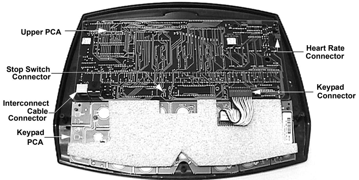
8. Remove the interconnect cable from its retaining clip, See Diagram 5.1. Holding the display housing by the plastic portions, do not handle the upper PCA or keypad PCA, reconnect the interconnect cable to the upper PCA.
