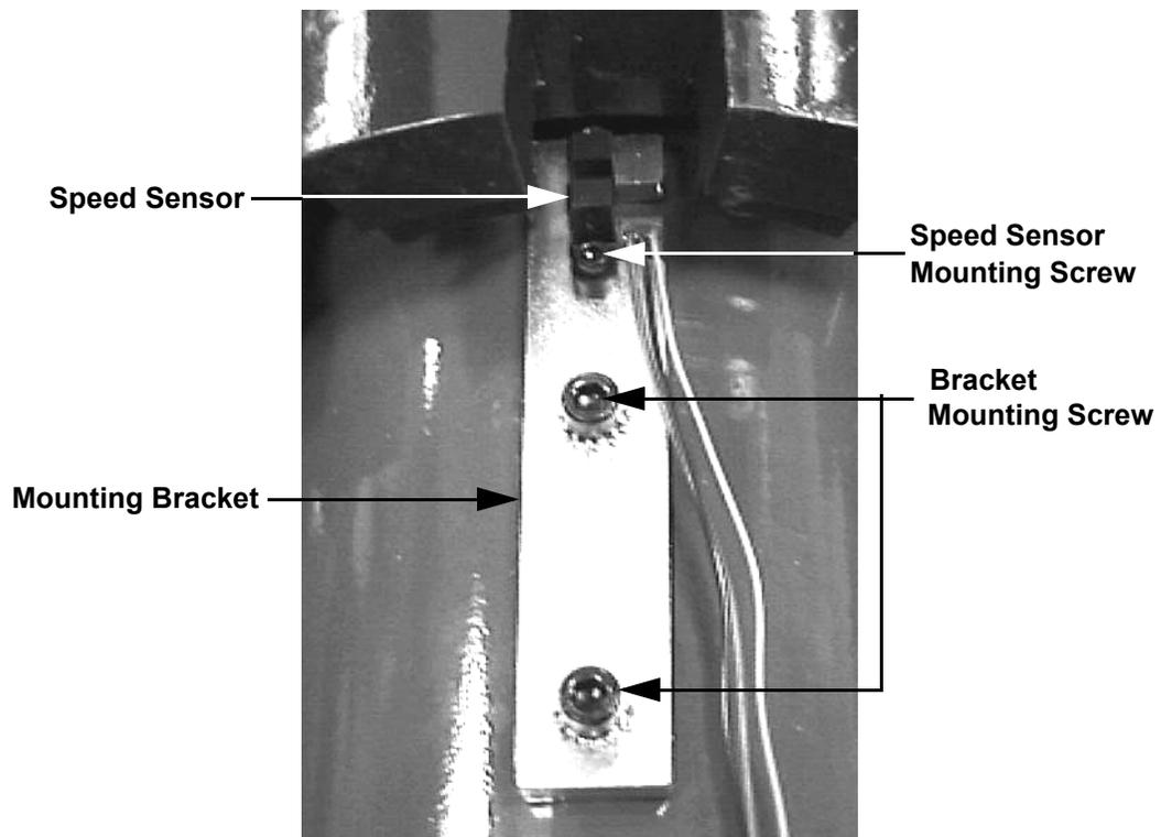
5. Remove the mounting bracket from the drive motor.
