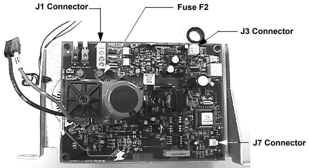
4. Insert the treadmill's line in the AC outlet and set the circuit breaker in the "on" position. Set the treadmill in the manual program and press the **LIFT ▲** key. If the lift motor operates normally, test treadmill operation per Section 3. If the lift motor still does not operate, retest the lift fuse per steps 2 & 3. If the fuse is open again, continue with step 13. If the fuse is good continue with step 5.
