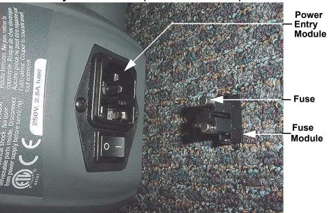
Diagram 7.24 - Power Entry Module Fuse (serial code AMPF)
