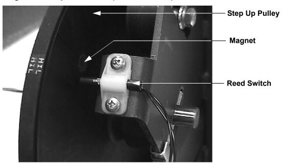
Diagram 6.4 - Speed Sensor (serial code AMPF)
