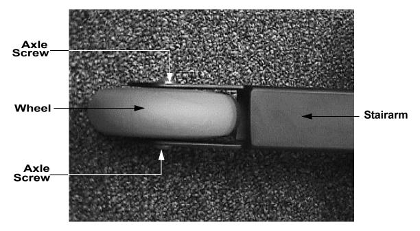
3. Set the replacement wheel in the stairarm and insert and hand tighten the wheel axle screws. Torque the wheel axle screws to 80 inch pounds.
