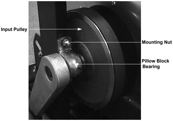
Diagram 7.10 - Pillow Block Bearings (serial code AMPF)
