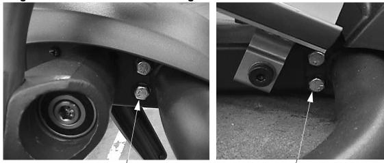
4. Remove the four bolts and washers that fasten the upper end of the frame tube to the main column. Remove the frame tube.
