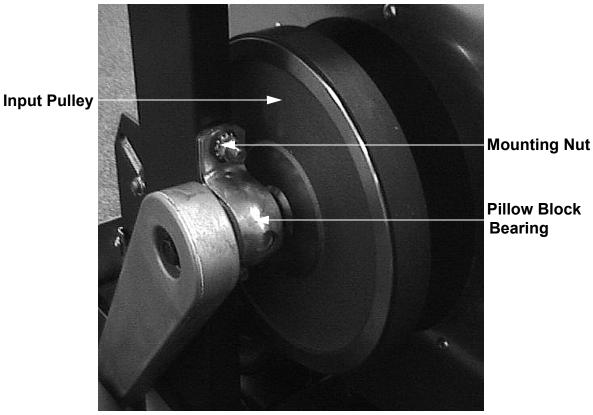
Diagram 7.10 - Pillow Block Bearings (serial code A998)
