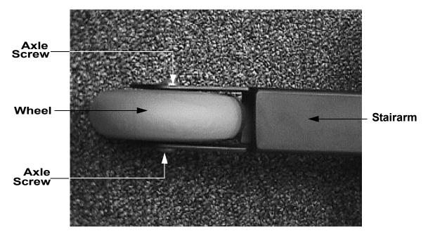
3. Set the replacement wheel in the stairarm and insert and hand tighten the wheel axle screws. Torque the wheel axle screws to 80 in/lbs.
