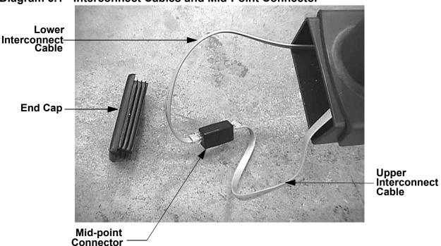
**Diagram 6.1 - Interconnect Cables and Mid-Point Connector**
