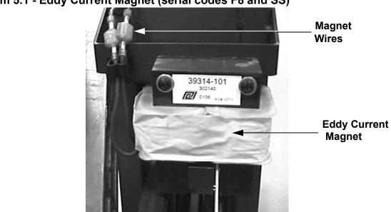
Diagram 5.1 - Eddy Current Magnet (serial codes F8 and SS)
