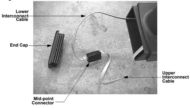
**Diagram 6.1 - Interconnect Cables and Mid-Point Connector**
