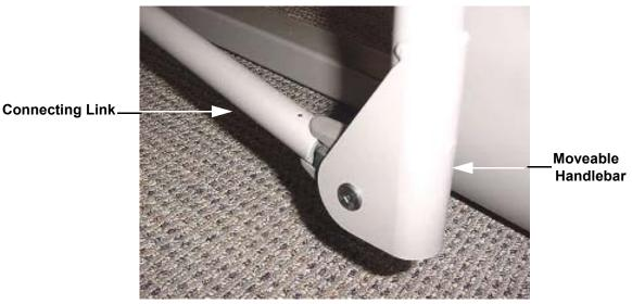
3. The rearward end of the connecting link will either be attached to the stairarm or to its storage point on the frame. Depress the orange button and remove the connecting link. Removing the connecting link prevents it from resting on the outrigger tube and will prevent the painted surfaces of the outrigger tube and connecting link from damage.
