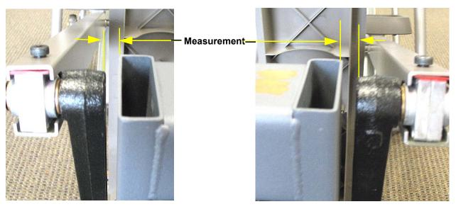
5. On the side with the larger measurement, loosen the upper pillow block mounting bolt only, do not loosen the lower pillow block mounting bolt. On the side with the smaller measurement, loosen both pillow block mounting bolts. See Diagram 5.7. For purposes of illustration we will assume that the left measurement was larger than the right side measurement in Diagram 5.6.
