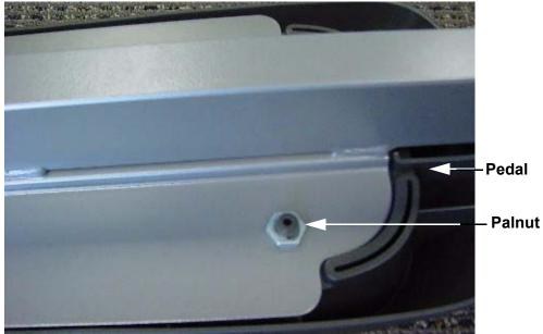
4. Set the pedal in its mounting position on the stairarm and fasten it with the four palnuts removed in step 2. The palnuts will cut new threads in the pedals plastic studs. Torque the palnuts to 6-9 inch pounds.
