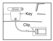
IMPORTANT: In an emergency, the key can be pulled from the console, causing the walking belt to slow to a stop. Test the clip by carefully taking a few steps backward; if the key is not pulled from the console, adjust the position of the clip. Note: The first time you insert the key into the console, the incline will automatically rise to the maximum incline level and then return to the minimum incline level.
