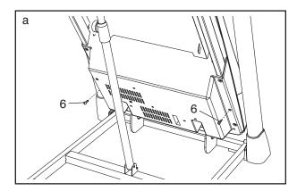
Next, remove the three indicated #8 x 3/4" Screws (6). Carefully slide the Motor Hood (57) off.
