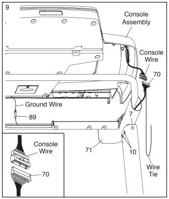
10. Set the console assembly on the Left and Right Handrails (71, 72). **Make sure that no wires are pinched.** Insert the excess Upright Wire (not shown) into the Left Handrail and the ground wires (not shown) into the console assembly.
