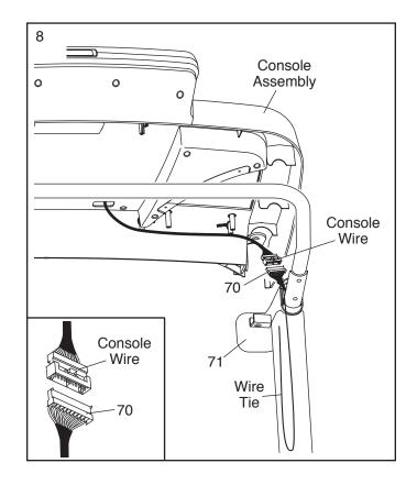
9. Set the console assembly on the Left and Right Handrails (71, 72). **Make sure that no wires are pinched.** Insert the excess Upright Wire (70) into the Left Handrail.
