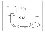
light. IMPORTANT: In an emergency, the key can be pulled from the console, causing the walking belt to slow to a stop. Test the clip by carefully taking a few steps backward; if the key is not pulled from the console, adjust the position of the clip.
