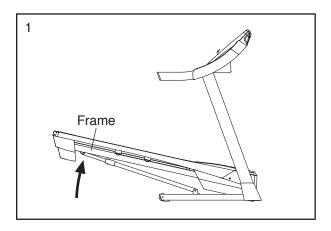
Raise the frame until the latch knob locks in the storage position. CAUTION: Make sure that the latch knob locks.
