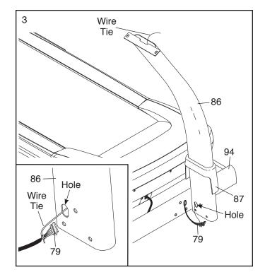
4. Hold the Upright (86) against the Base (94). **Be** careful not to pinch the Upright Wire (79). Insert three 3/8" x 2 3/4" Patch Bolts (7) with three 3/8" Star Washers (11) into the Upright.
