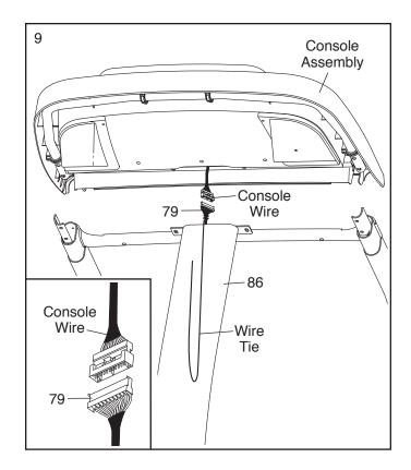
Set the console assembly on the Handrails (81, 82) and the Upright (86). Be careful not to pinch any wires. Insert the excess Upright Wire (not shown) into the Upright.
