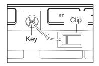
After a moment, the displays will light. IMPORTANT: In an emergency, the key can be pulled from the console, causing the walking belt to slow to a stop. Test the clip by carefully taking a few steps backward; if the key is not pulled from the console, adjust the position of the clip.
