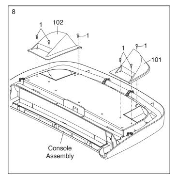
9. With the help of a second person, hold the console assembly near the Upright (86).
