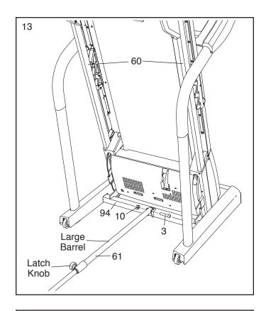
14. Attach the upper end of the Storage Latch (61) to the bracket on the Frame (60) with a 3/8" x 1 3/4" Patch Bolt (6) and a 3/8" Nut (10).
