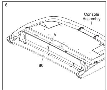
7. IMPORTANT: To avoid damaging the Crossbar (80), do not use power tools and do not overtighten the #10 x 3/4" Screws (8).
