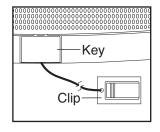
a moment, the displays will light. IMPORTANT: In an emergency situation, the key can be pulled from the console, causing the walking belt to slow to a stop. Test the clip by carefully taking a few steps backward; if the key is not pulled from the console, adjust the position of the clip.
