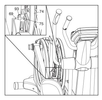
Next, rotate the Large Pulley (74) until a Magnet (75) is aligned with the Reed Switch (69). Slide the Reed Switch slightly toward or away from the Magnet. Then, retighten the M4 x 16mm Screw (93).
