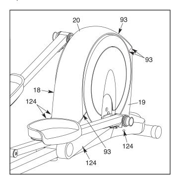
Next, remove the M4 x 16mm Screws (93) and the M4 x 42mm Screws (124) from the Right and Left Shields (18, 19). **Make sure to note which size of Screw you remove from each hole.** Then, gently remove the Left Shield.
