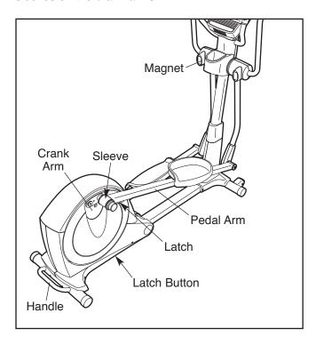
Next, raise the pedal arms until they touch the magnets on the upper body legs; the magnets will hold the pedal arms in place. Then, hold the handle and lift the frame until it locks in a vertical position.
