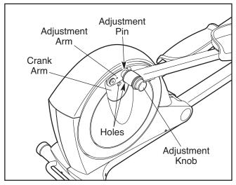
Pivot the adjustment arm back and forth slightly to make sure that the adjustment pin is engaged in one of the holes in the crank arm.
