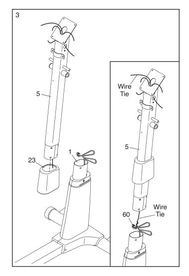
4. **Tip: Avoid pinching the Wire Harness (60).** Insert the Upright (5) into the Frame (1).
