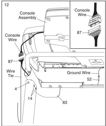
13. Set the console assembly on the Left and Right Handrails (82, 83). **Be careful not to pinch any wires.** Insert the excess Upright Wire (87) into the Right Handrail.
