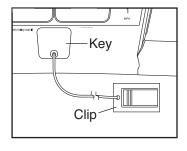
IMPORTANT: In an emergency, the key can be pulled from the console, causing the walking belt to slow to a stop. Test the clip by carefully taking a few steps backward; if the key is not pulled from the console, adjust the position of the clip.
