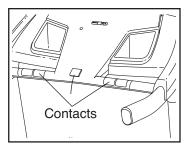
To use the handgrip heart rate monitor, stand on the foot rails and hold the metal contacts—avoid moving your hands. When your pulse is detected, your heart rate will be shown. For the most accurate heart rate reading, continue to hold the contacts for about 15 seconds.
