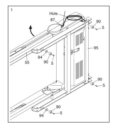
2. **See the inset drawing.** Cut the plastic tie near the Upright Wire (87).
