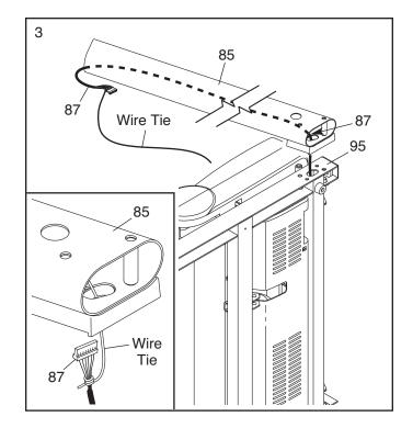
Hold the Right Upright (85) against the Base (95). Be careful not to pinch the Upright Wire (87). Insert two 3/8" x 4" Screws (7) and a 3/8" x 1 1/2" Screw (3) with three 3/8" Star Washers (11) into the Right Upright.
