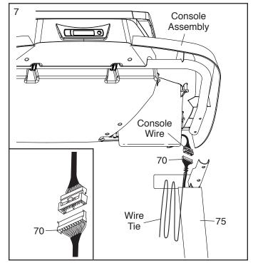
8. Set the console assembly on the Handrails (71). **Be careful not to pinch any wires.** Insert the excess Upright Wire (70) into the Left Upright (75).
