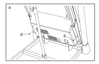
Lower the treadmill (see HOW TO LOWER THE TREADMILL FOR USE on page 22). Remove the five #8 x 3/4" Screws (6). Carefully slide the Motor Hood (57) off.
