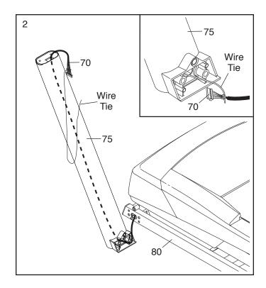
3. With the help of a second person, hold the Left Upright (75) against the Base (80). **Be careful not to pinch the wires.**
