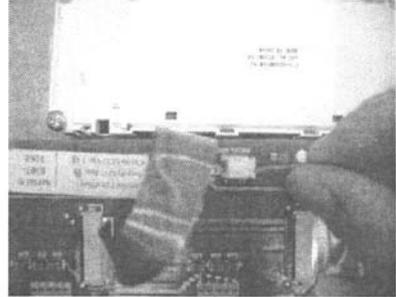
4) Next plug in the backlight from the LCD to the upper display board. This plug will only go in one way.
