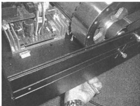
7. Slide drive-belt off drive motor flywheel.
