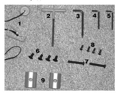
**Step 1:** Carefully unpack treadmill and check that all hardware is present as shown.
