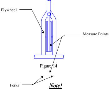
Do not over tighten the nut on the end of the axle. This will result in breaking off the end of the axle or stripping the axle threads. 35 ft-lbs. is equivalent to applying 35 lbs. of weight or force to the end of a 12 inch long wrench. Also make sure to remove chain adjustment tool.
