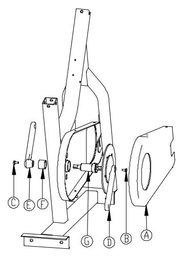
7. Using splined bottom bracket socket, remove the bottom bracket cartridge 'G' and discard. *The cartridge* 'G' is *left-hand threaded meaning you turn the tool clockwise to remove the cartridge*.
