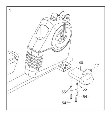
While another person lifts the rear of the Frame (1), attach the Rear Stabilizer (16) to the Frame with four M8 x 55mm Patch Screws (52) and four M8 Split Washers (55).
