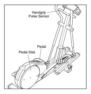
To dismount the elliptical crosstrainer, wait until the pedals come to a complete stop. The elliptical crosstrainer does not have a free wheel; the pedals will continue to move until the flywheel stops. When the pedals are stationary, step off the highest pedal first. Then, step off the lowest pedal.
