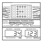
the + button (this is the button that also selects resistance level 10). While an E or an M appears in the matrix, the left display will show the total numbers of hours that the elliptical crosstrainer has been used, and the right display will show the total number of miles pedaled. When you are finished viewing this information, press the Start Program button again.
