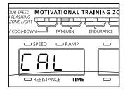
CAL will appear in the left display and the indicators in the Training Zone bar will flash in sequence. Calibration will last one to two minutes.
