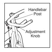
Make sure that the adjustment knob is engaged in an adjustment hole in the handlebar post.
