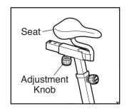
Make sure that the adjustment knob is engaged in an adjustment hole in the seat carriage.
