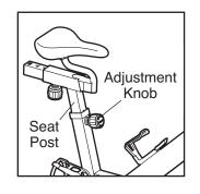
that the adjustment knob is engaged in an adjustment hole in the seat post.
