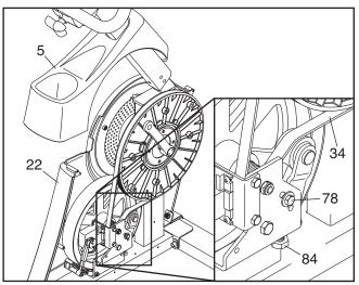
Then, remove all the screws from the Left and Right front shields (22, not shown); **there are three sizes of screws in the Front Shields—note which size of screw you remove from each hole.** Then, gently pull the Right Front Shield away from the frame.
