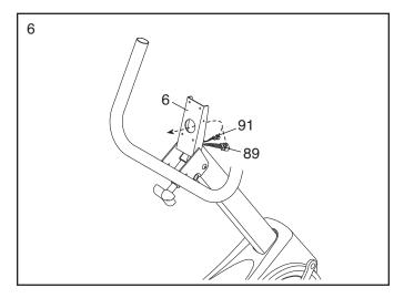
While another person holds the Console (7) near the Handlebar (6), connect the wires on the Console to the Wire Harness (89) and the Frame Pulse Wire (91).
