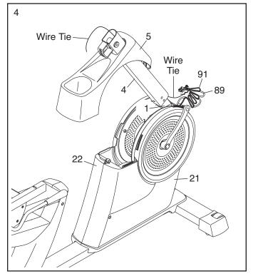
5. Make sure that the Wire Harness (89) and the Frame Pulse Wire (91) are in the location shown.
