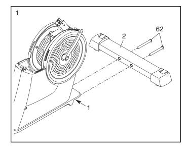
While another person lifts the rear of the Frame (1), attach the Rear Stabilizer (3) to the Frame with two M10 x 95mm Patch Screws (62).
