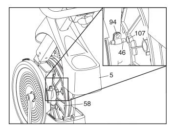
Locate the Reed Switch (46). Turn the Pulley (58) until a Magnet (107) is aligned with the Reed Switch. Next, loosen, but do not remove, the indicated M4 x 13mm Flange Screw (94). Slide the Reed Switch slightly closer to or away from the Magnet, and then retighten the Screw. Turn the Pulley for a moment. Repeat these actions until the console displays correct feedback. When the reed switch is correctly adjusted, reattach the shield cover.
