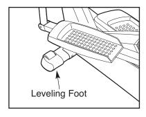
rocks slightly during use, turn one or both of the leveling feet under the front stabilizer until the rocking motion is eliminated.
