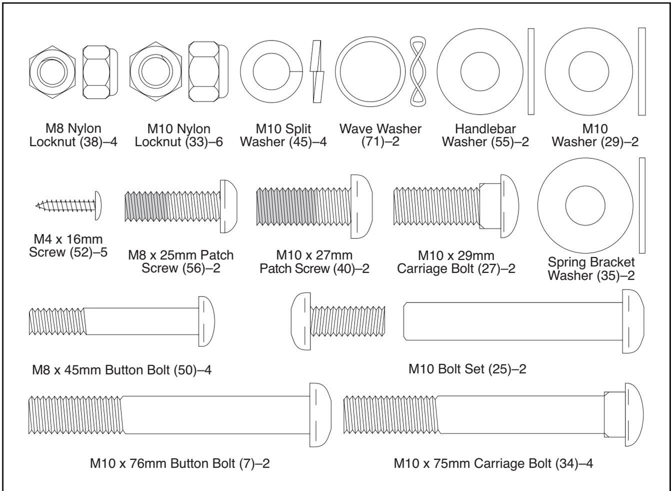
1. Identify the Front Stabilizer (10), which has round Endcaps (21). While another person lifts the front of the Frame (1), attach the Front Stabilizer to the Frame with two M10 x 75mm Carriage Bolts (34) and two M10 Nylon Locknuts (33).
