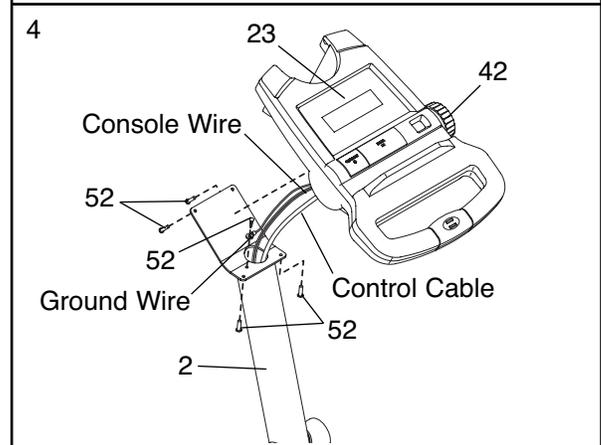
Attach the Console (23) to the Upright (2) with four M4 x 16mm Screws (52). **Be careful to avoid pinching the cable and wires.**
