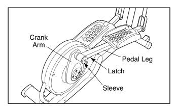
Next, raise the pedal legs until they touch the magnets on the upper body arms; the magnets will hold the pedal legs in place. Then, hold the handle and lift the frame until it locks in a vertical position.
