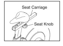
an adjustment hole in the seat carriage, and firmly tighten the seat knob. Make sure that the seat knob is engaged in an adjustment hole.
