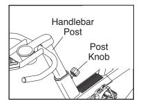
in the handlebar post, and firmly tighten the post knob. Make sure that the post knob is engaged in an adjustment hole.
