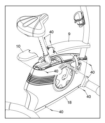
Remove the five M4 x 16mm Screws (40) from the Right Shield (18). Then, gently move the Right Shield away from the frame.
