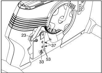
Then, reattach the right shield, the top shield, and the top shield cap. Reattach the right pedal, if necessary.
