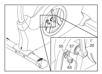
Next, rotate the Left Crank Arm (20) until a Magnet (55) is aligned with the Reed Switch (57). Slide the Reed Switch slightly toward or away from the Magnet. Then, retighten the M4 x 13mm Flange Screws (63).
