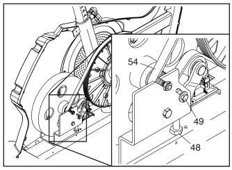
When the Drive Belt (54) is tight, tighten the M6 x 20mm Hex Screw (49).
