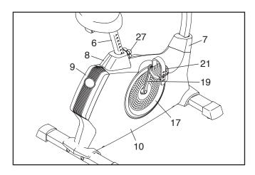
Next, remove the Seat Post Knob (27) and remove the Seat Post (6).
