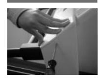
Place the plastic endcaps on the top corners of the control panel. Use the two small Phillips head screws included to secure the endcaps.
