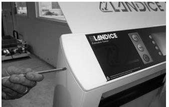
Align the side frame cover beneath the end cap and install the <u>Phillips</u> head screw.
