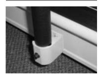
Fit the side rail clamp to the bottom side frame at the hole provided. Use a 5/16" wrench to hold nut inside treadmill and use 3/16" allen wrench to tighten.
