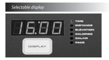
The **DISPLAY** button allows you to move about the selectable display. You can move the selectable display automatically from option to option by using the Scan mode. Press and hold the **DISPLAY** button for 3 seconds to enter the Scan mode. When in the Scan mode the display will advance by itself every five seconds. Press the **DISPLAY** button one more time to exit the Scan mode.
