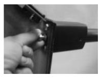
Insert the side rail into the upper rail clamp and tighten the bolt using a 1/2" socket. (*Do not over-tighten.*)
