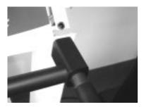
Insert the side rail into the upper rail clamp.
