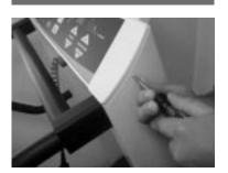
Place the plastic endcaps on the top corners of the control panel. Use the two small Phillips head screws included to secure the endcaps.
