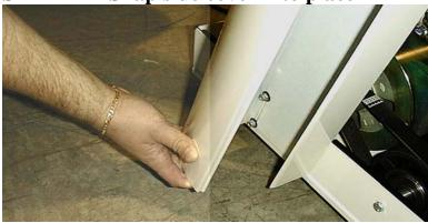
Carefully align the side frame cover. Working from top to bottom, snap the upright side cover into place.
