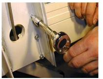
Slide the upright down onto the 8 side frame bolts. Be sure the washers are located on the outside of the upright and against the head of the bolt. Tighten bolts with a 3/8" extended socket.
