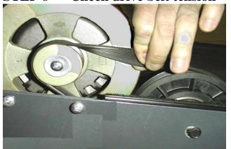
Check the tension on the drive belt by placing the drive belt between your thumb and forefinger and twisting.
