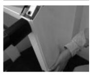
Carefully align the side frame cover. Working from top to bottom, snap the upright side cover into place
