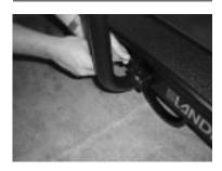
Use a 3/16" allen wrench to tighten the rail clamp bolts.
