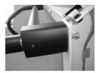
Attach the medrail by first handstarting the bolts and then using a 1/2" socket until snug. (*Do not over-tighten*.)
