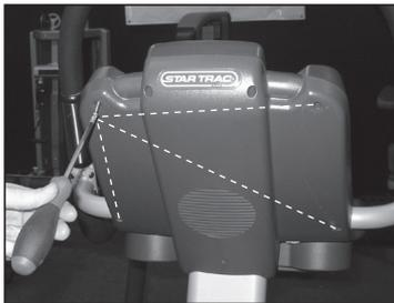
Remove the four screws from the display.
