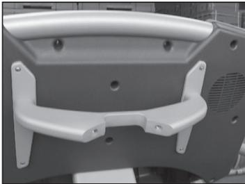
Attach the crossbow to the wings and leave the nuts slightly loose so you can position them onto the display, do not attach the back of the crossbow at this time.
