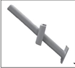
Slide the top mounting plate on the neck and align the top plate notch with the neck base notch.
