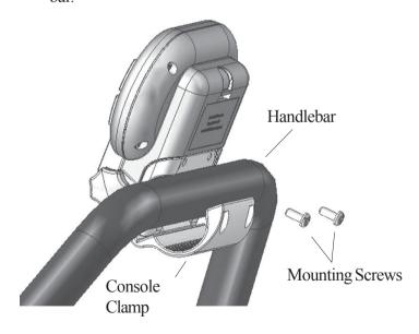
3. Insert a mounting screw into each hole and use a 4-mm hex key to tighten the screws.
