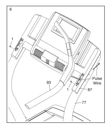
7. Set the Right Handrail Assembly (93) onto the right Upright (77). **Make sure that no wires are pinched.**
