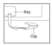
console to be ready for use. IMPORTANT: In an emergency, the key can be pulled from the console, causing the walking belt to slow to a stop. Test the clip by carefully taking a few steps backward; if the key is not pulled from the console, adjust the position of the clip.
