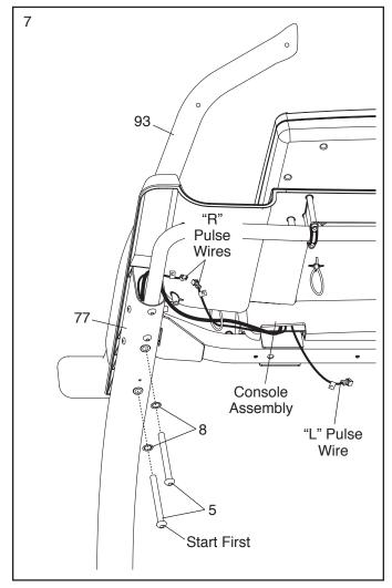
Hold the Left Handrail Assembly (86) near the left Upright (77). Insert the pulse wire from the left handrail assembly into the hole in the top of the Upright and pull it out of the end of the Upright.
