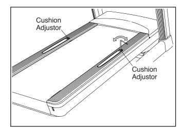
To decrease the firmness, step off the treadmill and use a hex key to turn the cushion adjustors counterclockwise 1/4 turn until the word "On" appears next to the cushion adjustor.
