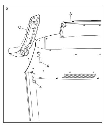
Tighten a #8 x 1/2" Screw (10) and a #8 x 3/4" Screw (5) into the console assembly and the right handrail assembly (C) in the locations shown. Do not overtighten the Screws.
