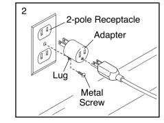
tending from the adapter must be connected with a metal screw to a permanent ground such as a properly grounded outlet box cover. Some 2-pole receptacle outlet box covers are not grounded. Before using an adapter, contact a qualified electrician to determine whether the outlet box cover is grounded. The temporary adapter should be used only until a properly grounded outlet can be installed by a qualified electrician.
