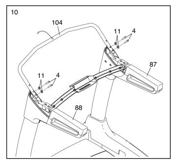
11. With the help of a second person, hold the console assembly near the Left Handrail (88).
