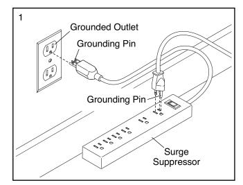
A temporary adapter may be used to connect the surge suppressor to a 2pole receptacle if a properly grounded outlet is not available. The lug or wire ex-
