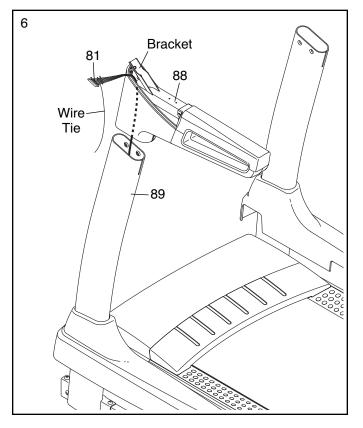
Attach the Left Handrail (88) to the Left Upright (89) with two 5/16" x 1" Screws (5) and a 5/16" x 1 1/2" Bolt (4). Do not fully tighten the Screws and the Bolt yet.
