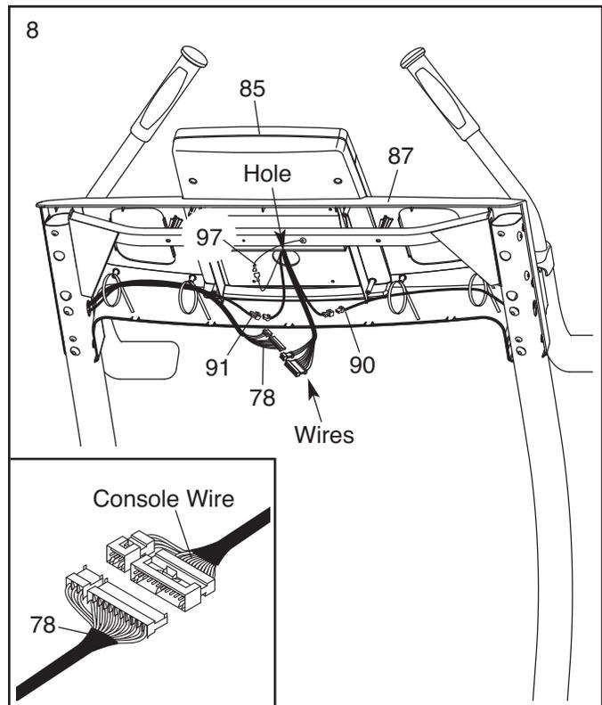
9. Attach the Console (85) with four #8 x 3/4" Screws (1). **Start all four Screws, and then tighten each of them. Do not overtighten the Screws.**
