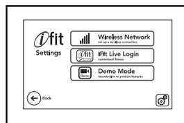
You must have your own wireless network and an 802.11b router with SSID broadcast enabled (hidden networks are not supported).
