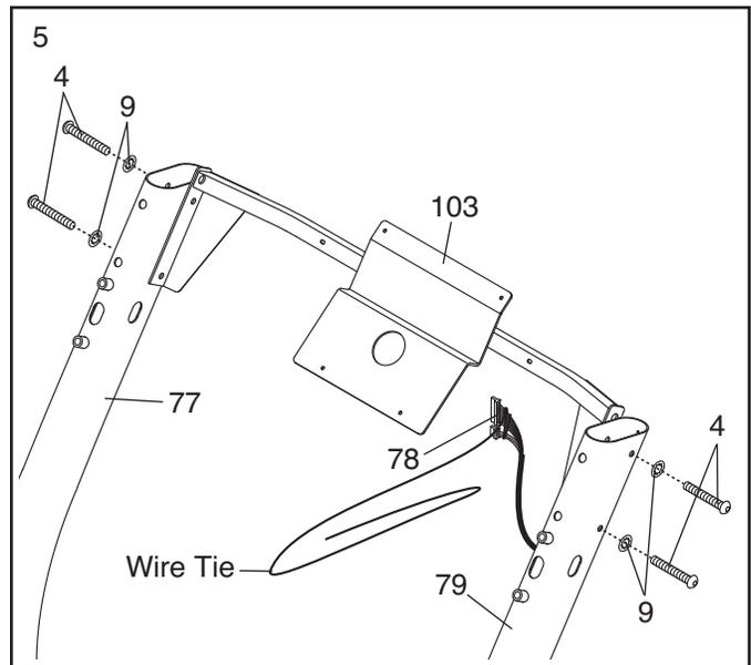
6. Set the Console Cover (87) on the Uprights (77, 79). Make sure that the Console Cover is oriented with the ties toward the bottom as shown.
