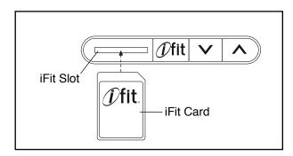
Next, select the desired workout on the iFit card by pressing the increase and decrease buttons next to the iFit slot.
