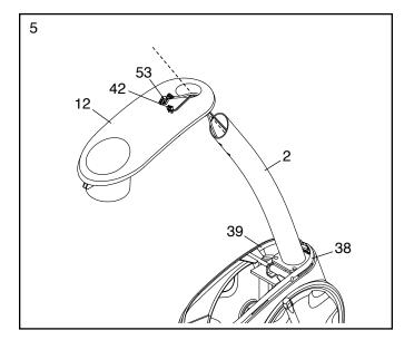
Orient the Console Plate (11) as shown. Then, insert the Main Wire (53) and the Frame Pulse Wire (42) upward through the Console Plate.
